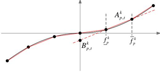
Fig. 2. Piecewise linear approximation of pipeline flow.
